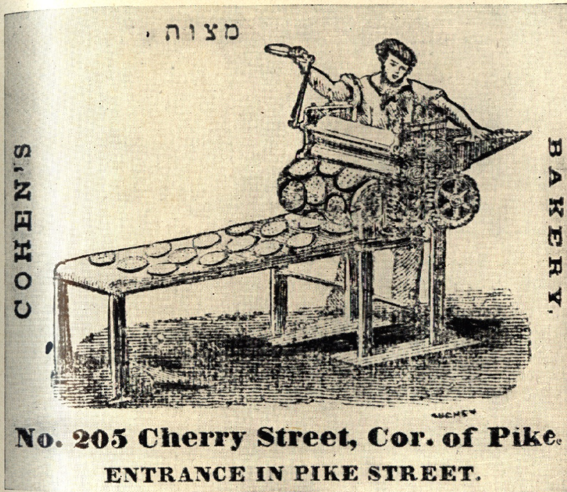
A Crude Drawing of an Early Matzoh Machine 1855
